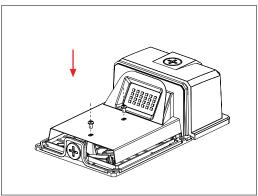
8. Screw down the reflector with screws.
