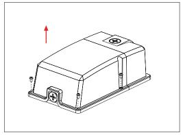
1. Use screwdriver to remove the screws of fixture 2. Use screwdriver to remove the reflector cover, and then take down the cover.
