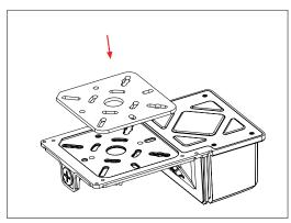
4. Attach the gasket to the back shell. Attention: the hole on both should be matched.
