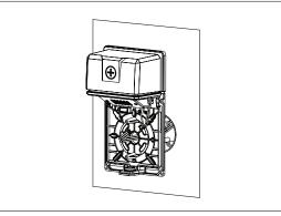
5. Pass the input line in the junction box through the waterproof gasket and then pass it through the fixture base.
