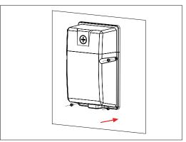
9. Use screws to tighten up the fixture, then installation completed.
