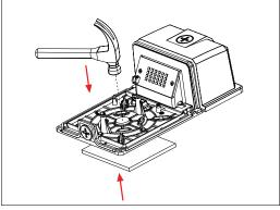
3. Put the gasket on the concave side of the fixture. It is used to avoid the damage of back shell when it struck by hammer. Then hammer the plugs of the cable entry and mounting hole.
