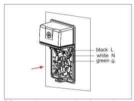
7. Connect the fixture input line, then put the connected wires into the embedded junction box.
