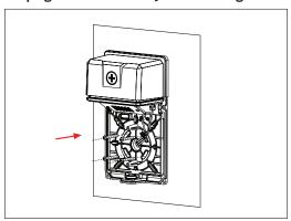
6. Lock the fixture base with the screw on the embedded junction box.
